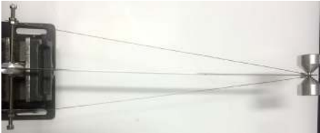
FIGURE 10: Experimental setup for finding natural frequencies for one pair of cables.
