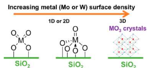
Figure 2. Proposed structures of the \text{MO}_x species on the \text{SiO}_2 surface ( M = \text{Mo} or \text{W} ). Dioxo (\text{O}=\text{O})_2\text{MO}_2 , mono-oxo \text{O}=\text{MO}_4 , and species coexist with crystalline \text{MO}_3 .
