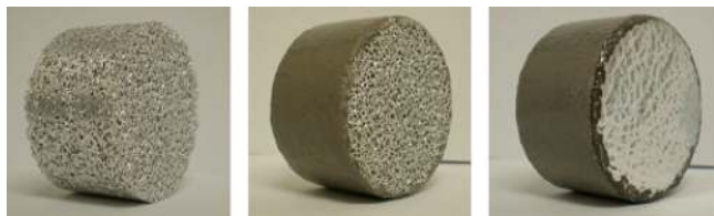
FIG. 5. (Color online) (a) Aluminum foam sample (left), (b) Sample's side coated with epoxy (center), and (c) Sample's face covered with aluminum tape (right).
