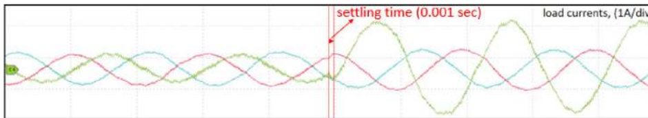
FIGURE 26 Results with phase unbalance in the reference and step change in the load with the proposed method at an AC frequency f_s = 50 Hz
