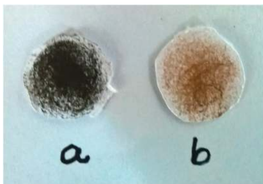
Scheme 1 Photographic image for the zero valent iron nanoparticles changing their color from (a) black to (b) brown after exposure to moisture (images were taken by placing the samples on a white paper).
