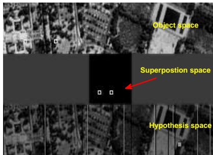
Fig. 8. ( Media 1 ) showing error in decoding two targets with the same velocity, the same y-coordinate, and with a separation which is an element of set \mathbf{S}_2 . Correct decoding is possible only when the targets begin to differ in their velocities. (Movie size: 0.9 MB)
