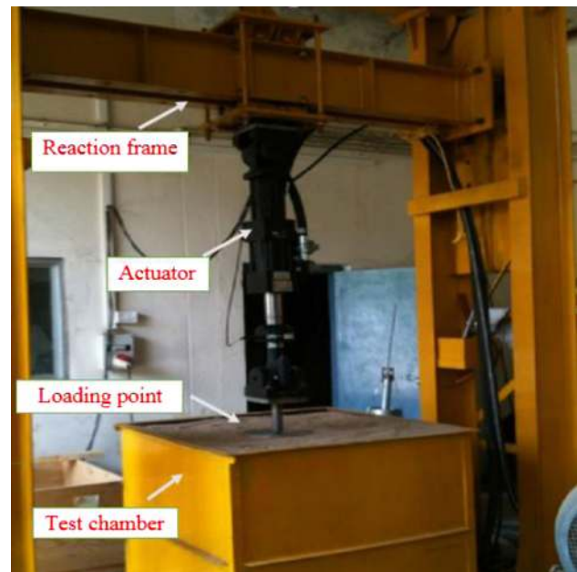
Fig. 4 Photograph of the test frame, test chamber, and actuator
