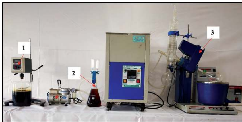
Fig. 1 Overhead-stirring upgradation strategy (1 – blending of CTPO, silica gel, and petroleum ether using a lab stirrer in 6 L glass beaker, 2 – Millipore filtration system, 3 – evaporation system coupled with low temperature cryostat bath and vacuum pump).
