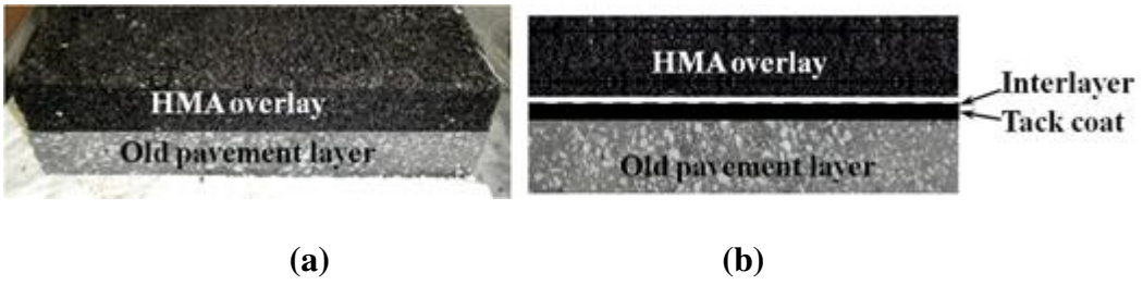
Fig. 1: a) Photograph and b) schematic of two-layer asphalt concrete beams
