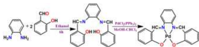
Scheme 1. Synthetic routes for the Schiff base and palladium complex 1 formulation.
