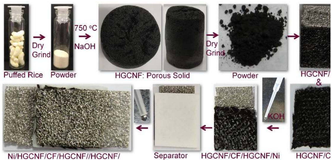
Scheme 1. Photographs illustrating the step-wise fabrication of the symmetric Ni/HGCNF/CF/HGCNF//HGCNF/CF/HGCNF/Ni cell starting from the bio-resource, puffed rice.
