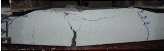
(a) Control Beam (Flexure-Shear Mode)
