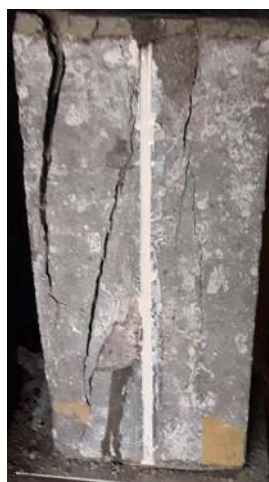
(iii) Pre-damaged and NSM strengthened
