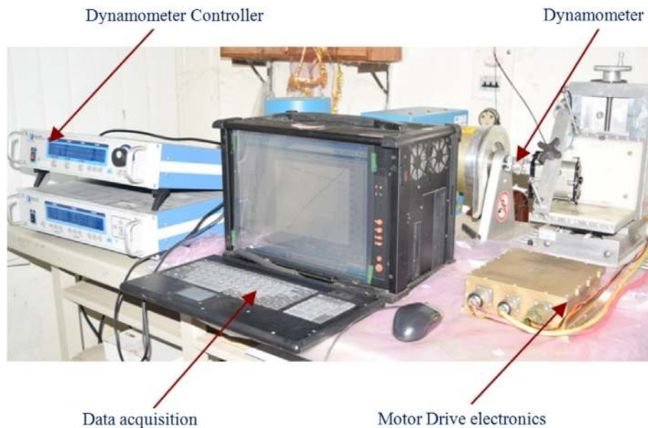
FIGURE 18 Experimental set-up of Halbach BLDC motor
