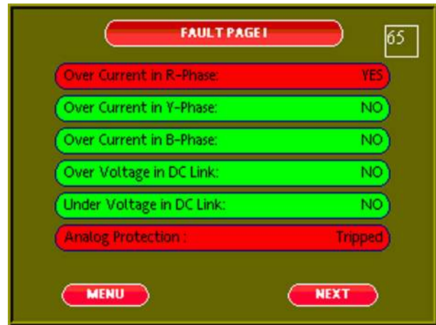
Figure 5. Fault annunciation in the HMI.
