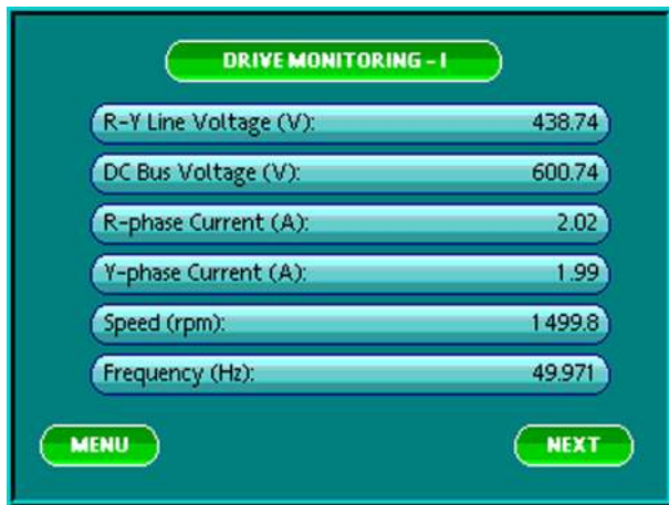
Figure 7. Parameter monitoring during RUN sequence.
