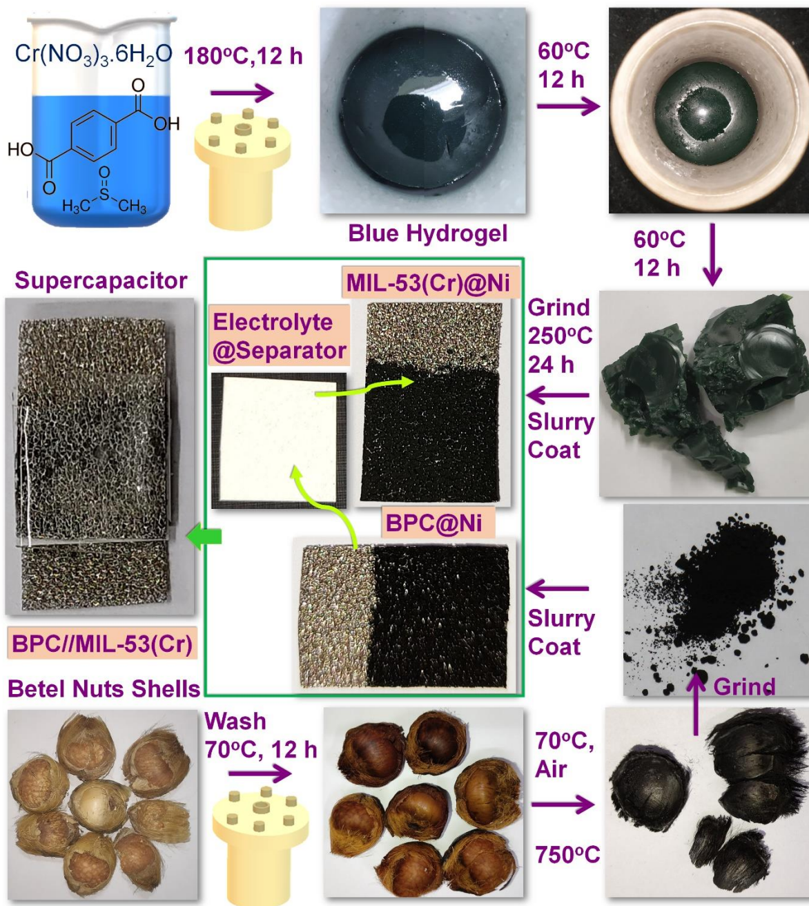
Scheme 1. Step-wise synthesis of MIL-53(Cr)-MOF and BPC and fabrication of their electrodes and full cell, is shown through photographs and cartoons.
