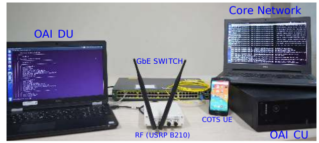
Fig. 4: OAI based NG-RAN testbed for different splits of NG-RAN.
