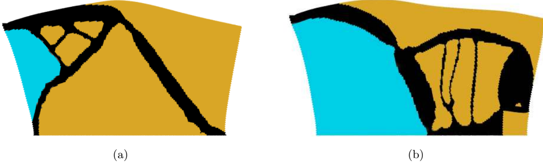
Figure 16: Deformed profiles for inverter and gripper mechanisms are displayed in (a) and (b) respectively.
