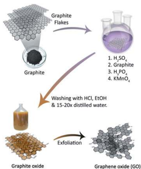
Fig. 1 Schematic of the synthesis process of GO (synthesis and exfoliation) starting from commercial graphite.
