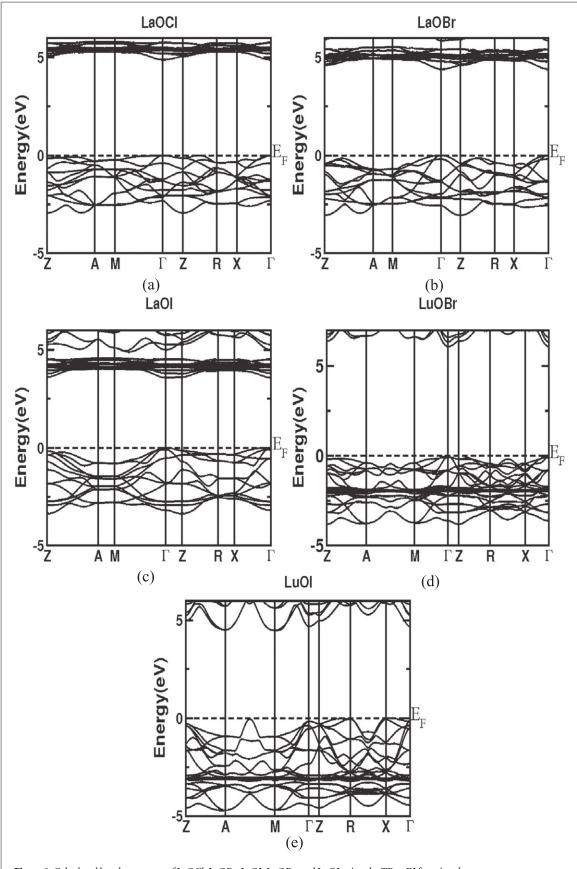
$\textbf{Figure 1.} \ Calculated \ band \ structures \ of \ LaOCl, \ LaOBr, \ LaOI, \ LuOBr, \ and \ LuOI \ using \ the \ TB-mBJ \ functional.$
