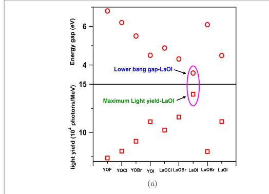
Figure 6. Energy gap and Maximum light yield values of LnOX (Ln = Y, La, Lu, and X = Cl, Br, I) compounds using the TB-mBJ functional.
