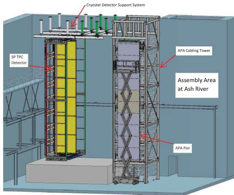
Figure 4.7. Phase 2 trial assembly at Ash River.
