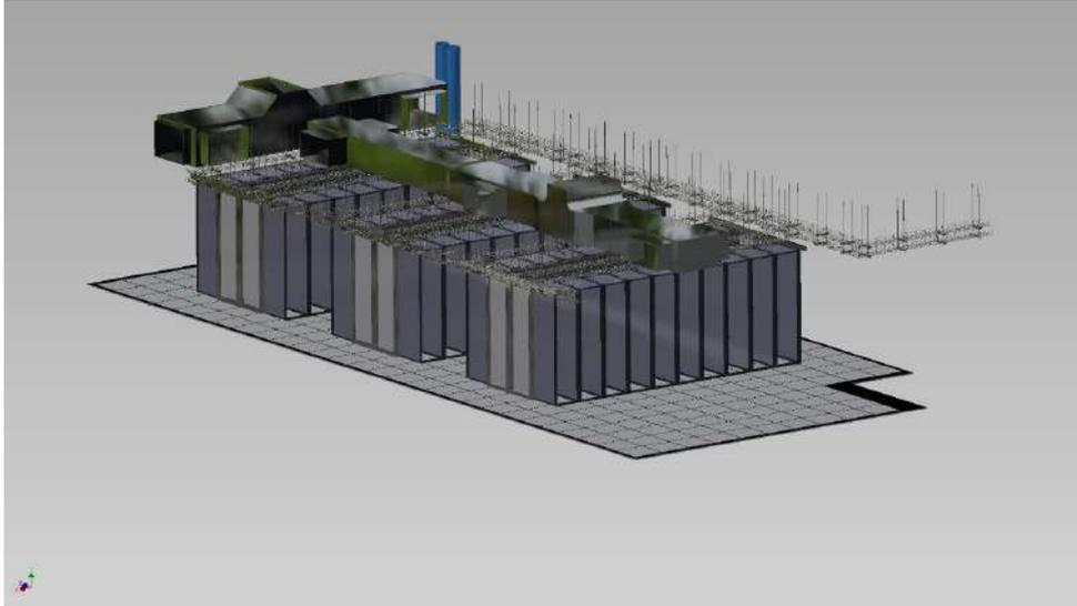
**Figure 5.16.** Proposed rack layout in DAQ room.
