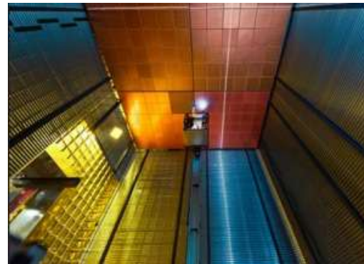
Figure 1.10. Left: view of one of the two drift volumes in ProtoDUNE-SP; the APA is on the left, the CPA is on the right, and two of the four the FC surfaces bounding the drift volume are at the center and bottom of the image. Right: the single ProtoDUNE-DP drift volume (still incomplete when the image was taken), looking up; the CRPs (orange) are at the top. Three sides of the surrounding FC are shown, but the cathode is not visible.
