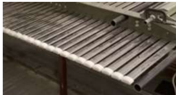
Figure 3.4. A section of the field cage, showing the extruded aluminum field-shaping profiles, with white polyethylene caps on the ends to prevent discharges.
