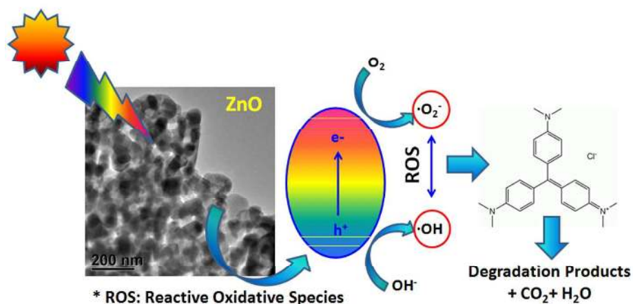
Figure 10: Schematic mechanism of ZnO as photocatalyst.
