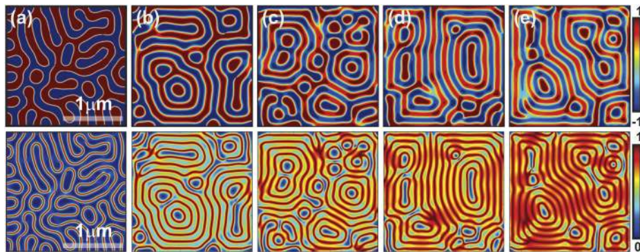
FIG. 4. Simulated domain (top) and domain wall (bottom) pattern with (a) original K_u and M_s , (b) 50% reduced K_u and original M_s , (c), (d) and (e) are having 50% reduced K_u with increase in M_s as 10%, 20% and 30% respectively. The scale bar is same for all the images.
