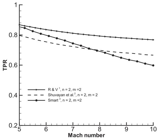
FIG. 2. Variation of total pressure recovery with Mach number.
