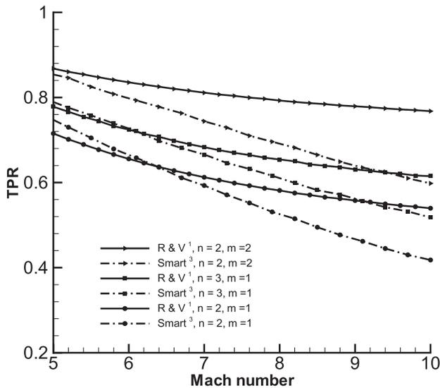
FIG. 1. Variation of total pressure recovery with Mach number.
