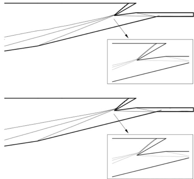
FIG. 3. Mach contours (min: 3.83, Δ: 0.65, and max: 7.08) for M = 8 geometry for constant specific heat (top) and variable specific heat (bottom).
