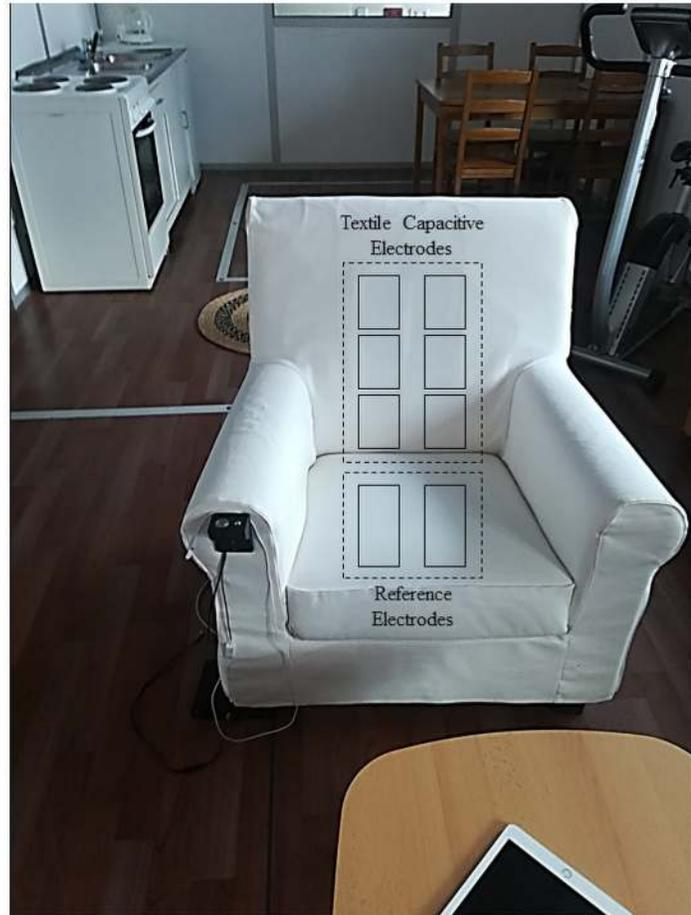
Fig 1. cECG armchair with capacitive electrodes.
