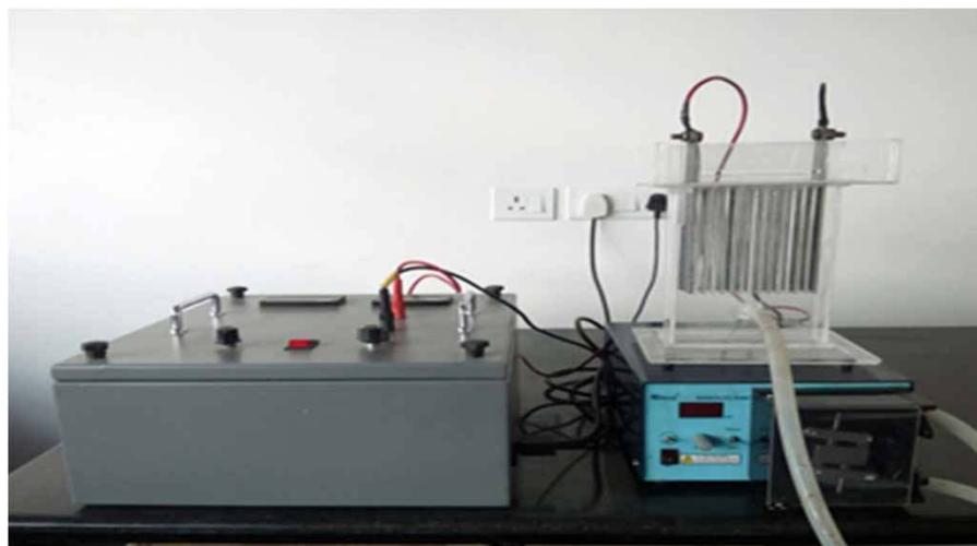
Figure 1 | Electrocoagulation set-up (1. DC power supply 2. CBME chamber 3. Peristaltic pump).
