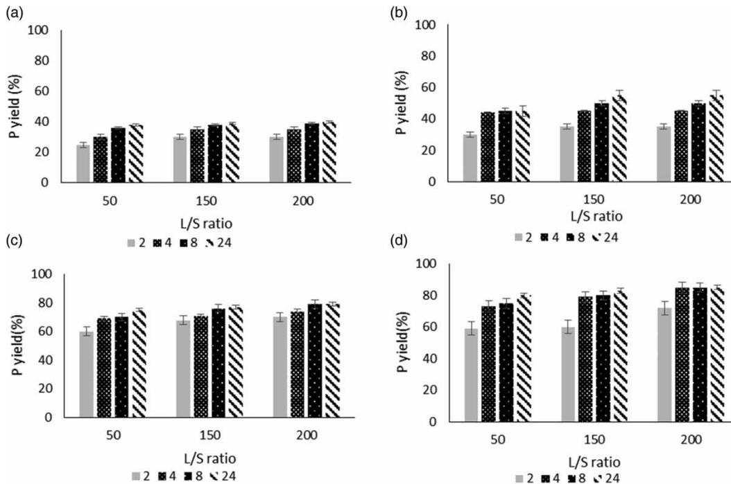
Figure 5 | Effect of liquid to solid ratio with sulphuric acid on sludge (a) Oven dried (b) Combustion at 600 °C (c) Combustion at 750 °C and (d) Combustion at 900 °C.
