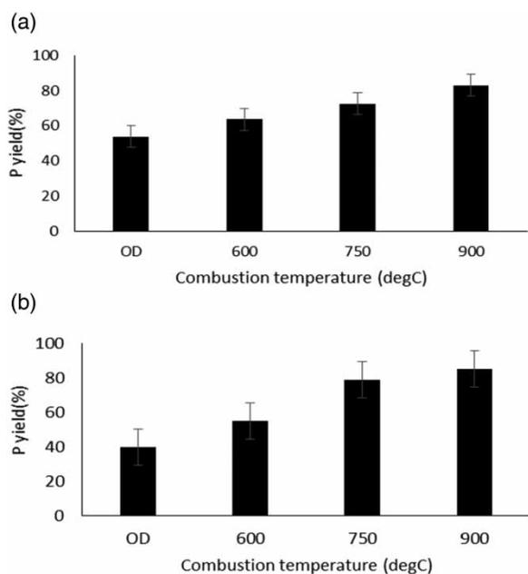
Figure 6 | Effect of combustion temperature (a) Oxalic acid (b) Sulphuric acid.
