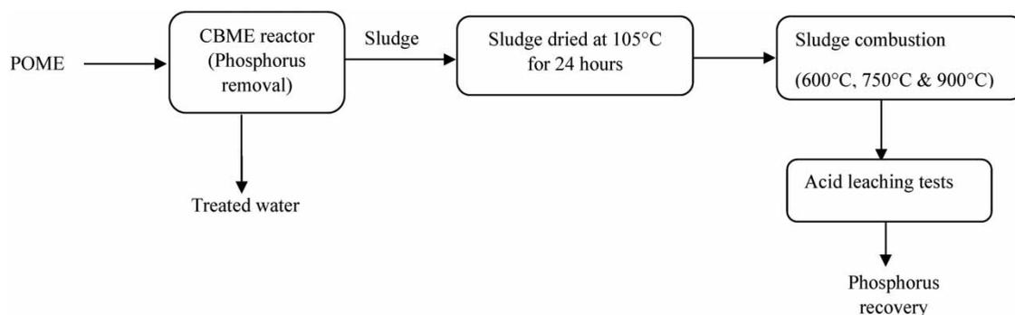
Figure 2 | Flow sheet of phosphorus recovery.
