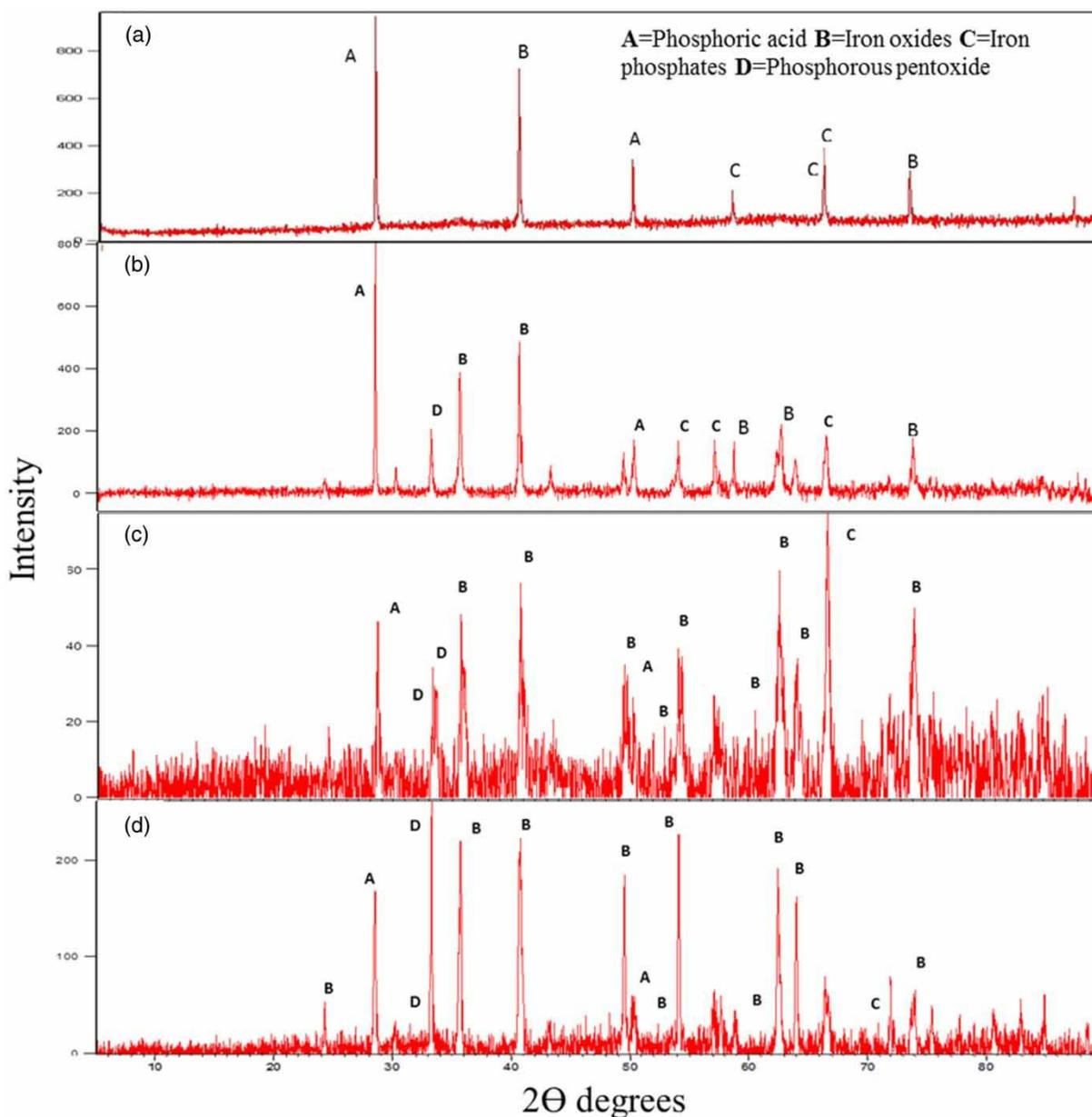
**Figure 3** | Sludge (a) Oven dried (b) Combusted at 600 °C (c) Combusted at 750 °C and (d) Combusted at 900 °C.
