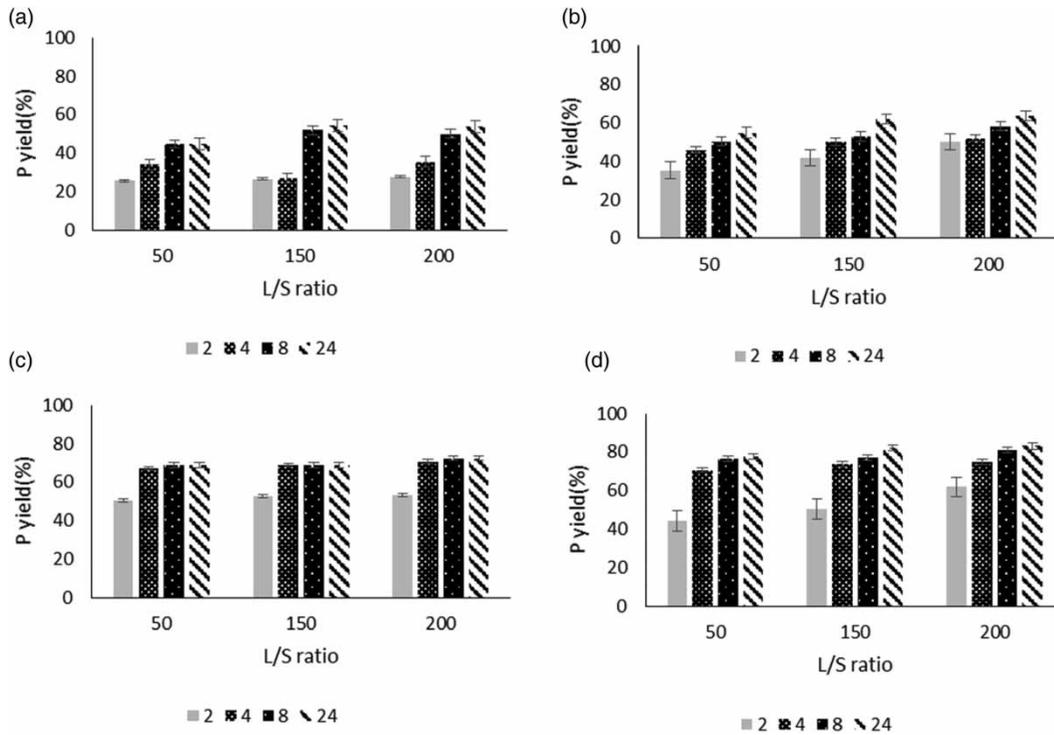
Figure 4 | Effect of liquid to solid ratio with oxalic acid on sludge (a) Oven dried (b) Combustion at 600 °C (c) Combustion at 750 °C and (d) Combustion at 900 °C.
