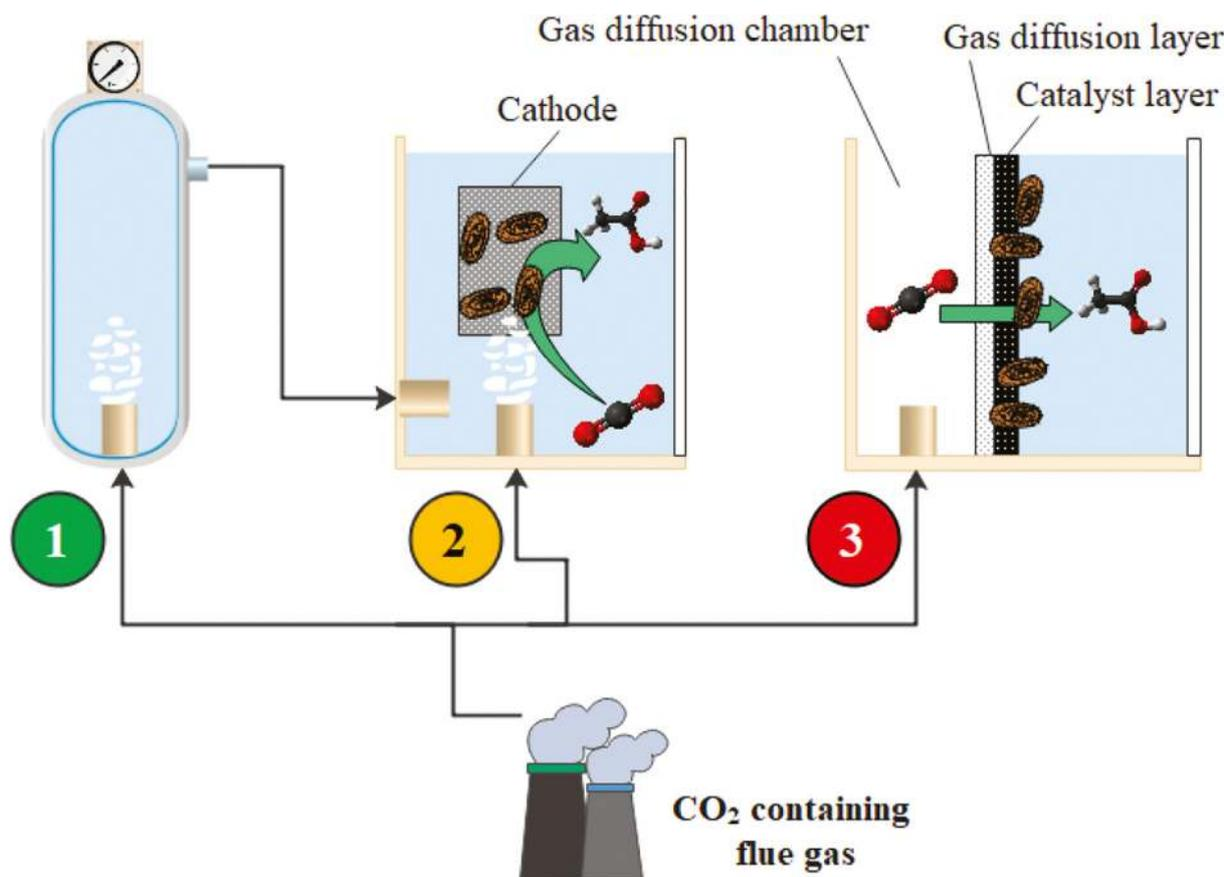
Fig. 5. CO<sub>2</sub> feeding strategies to MES reactors. CO<sub>2</sub> can be solubilised in a pressurised reactor and then delivered to the MES reactor (1), or directly delivered to the MES reactor through a sparger (2) or gas diffusion electrode (3).
