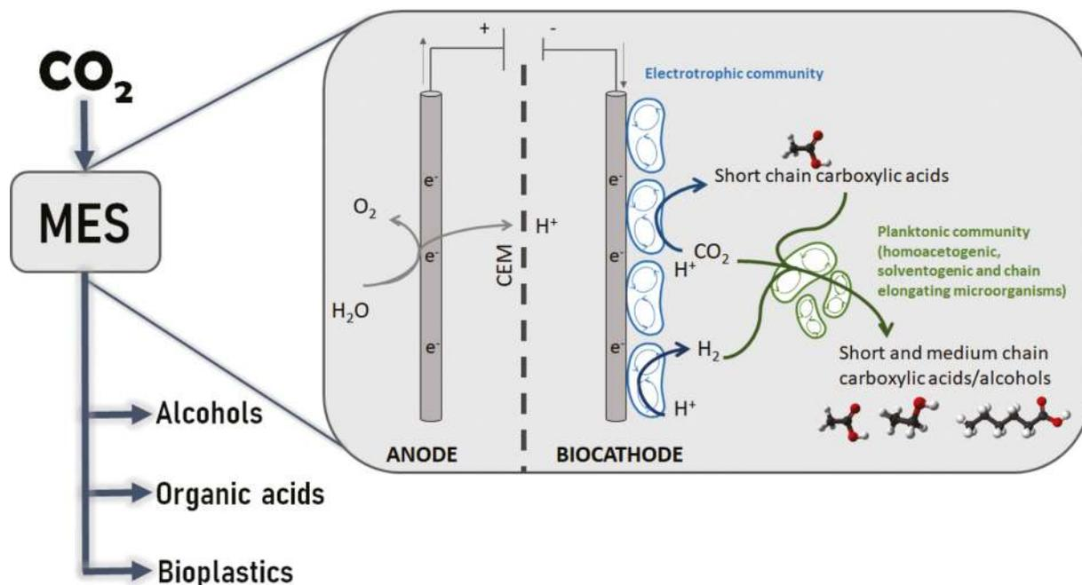
Fig. 1. Schematic representation of a typical MES configuration for biocommodities production from CO<sub>2</sub>.
