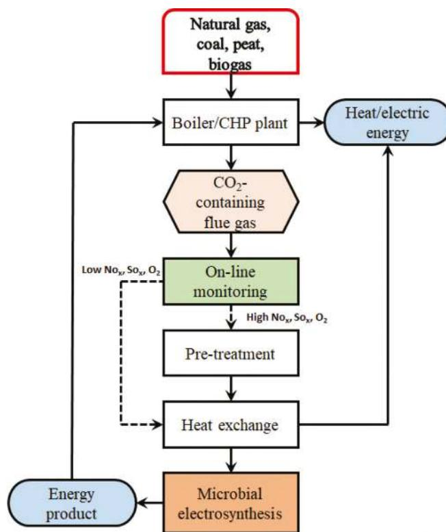
Fig. 3. Example of integration of MES for treatment of CO<sub>2</sub>-containing flue gas from the combustion of carbonaceous fuels. MES energy products (*e.g.* methane or alcohols) can be blended to the fossil fuels, further decreasing the carbon footprint of power plants.
