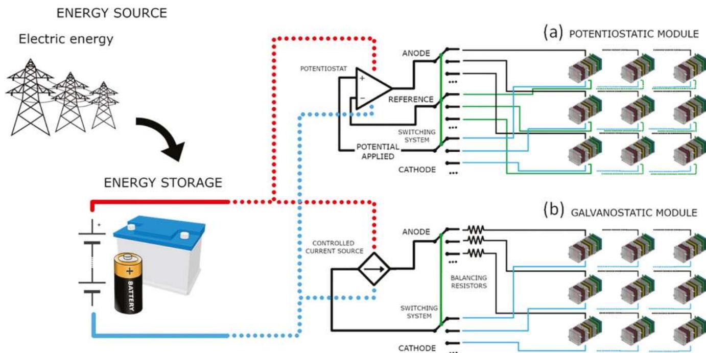
**Fig. 8.** Example of application of power managing system and smart electronics for potential or current control in MES stacks. (a) Each stack shares the same potential control amplifier which allows potential control in each cell through a multiplexer. (b) The cells are controlled in galvanostatic mode, and balancing resistors are connected in series to minimise differences among the cells. In case of failure, a stack can be switched off for maintenance without affecting the other stacks.
