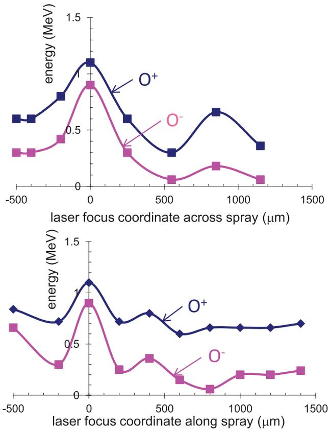
FIG. 4. (Color online) Ion energy dependence on laser focus position in spray. 0 is the centre of the spray defined with the accuracy of  $\pm 100 \mu\text{m}$ . The positive sign in the lower figure shows the direction of laser propagation.
