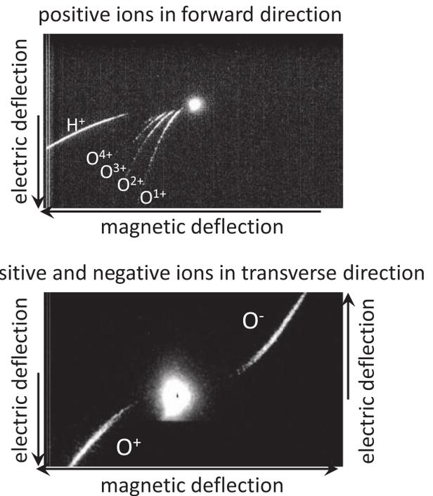
FIG. 3. Ion spectra in forward and transverse directions.
