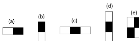
Figure 2. Kernels used to extract Haar-like features for the kidney detection algorithm. (a,b) Two-rectangle features. (c,d) Three-rectangle features and (e) Four-rectangle feature.
