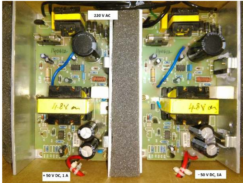
Figure 17. Power module designed for generating \pm 50 V DC.
