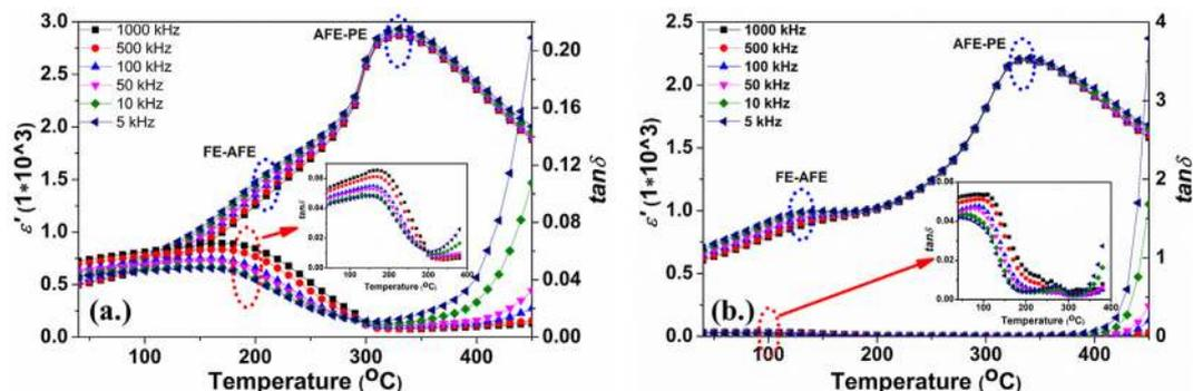
Fig. 6. Comparison of the dielectric constant in (a) NBT<sub>A</sub> and (b) NBT<sub>R</sub> samples as a function of temperature.
