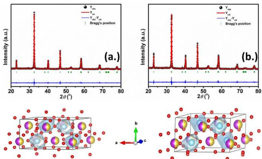
Fig. 3. Rietveld graphical output of (a)  $\text{NBT}_A$  and (b)  $\text{NBT}_R$  ceramics along with the monoclinic  $Cc$  phase drawn using VESTA package. The reflections position corresponding to the monoclinic phase is indicated by vertical bars.
