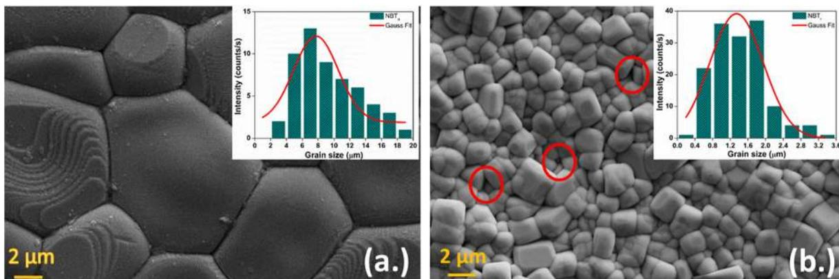
Fig. 4. Scanning electron micrographs of (a) NBT<sub>A</sub> and (b) NBT<sub>R</sub> ceramics.
