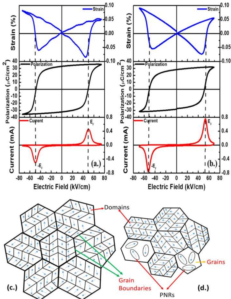
**Fig. 9.** Polarization-Electric ( $P$ - $E$ ) field, Current-Electric ( $I$ - $E$ ) field, and Strain-Electric ( $S$ - $E$ ) field loops of (a)  $NBT_A$  and (b)  $NBT_R$ . The schematic microstructure models of coarse-grained ( $NBT_A$ ) and fine-grained ( $NBT_R$ ) ceramics are shown in 9(c) and 9(d) depicting an increment in the domain walls elastic stiffness in  $NBT_R$  as compared to  $NBT_A$ .
