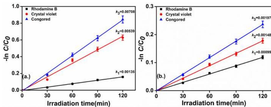
**Fig. 10.** First-order kinetics plots of (a) NBT<sub>A</sub> and (b) NBT<sub>R</sub>; exposure time-120 min, amount of catalyst –50 mgL<sup>-1</sup>, the concentration of dye - 50 ppm (The error bars indicate standard deviation).
