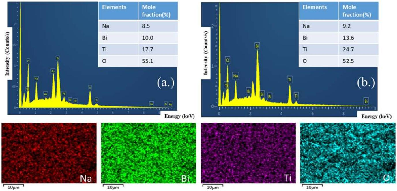
Fig. 5. SEM-EDS of (a) NBT<sub>A</sub> and (b) NBT<sub>R</sub> samples. Elemental mapping of NBT<sub>A</sub> sample.
