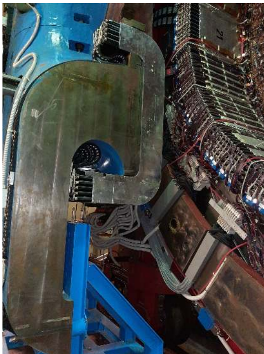
Figure 117. (left) A part of the KLOE magnet near one of the end caps. (right) The magnitude of the longitudinal (i.e., along the magnet symmetry axis) component of the magnetic field (in Gauss) as a function of the position along the magnet axis (in cm), measured from the center ( z = 0 cm) toward the end cap ( z \approx 200 cm). Data and MC are compared. The field was measured and simulated on the magnet symmetry axis.
