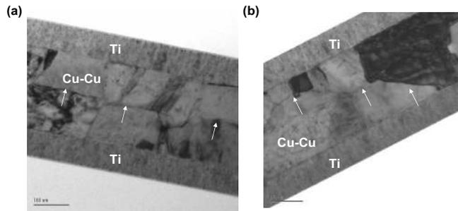
FIG. 4. TEM micrographs of bonded Cu layers: (a) without SAM passivation—only modest growth is observed and the original bonding interface can still be seen, and (b) with SAM passivation and desorption prior to bonding—substantial grain growth has taken place resulting in the formation of large Cu grains that extend beyond the original bonding interface.
