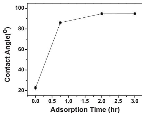
FIG. 1. Cu surface modification as a function of immersion time in SAM solution. Cu surface turns more hydrophobic and the contact angle value saturates beyond 2 h of immersion.
