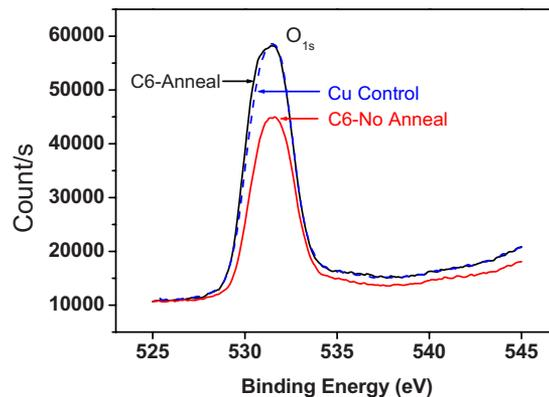
FIG. 3. (Color online) XPS data showing O content on wafer surface. SAM demonstrates the ability to protect Cu surface from excessive oxidation.
