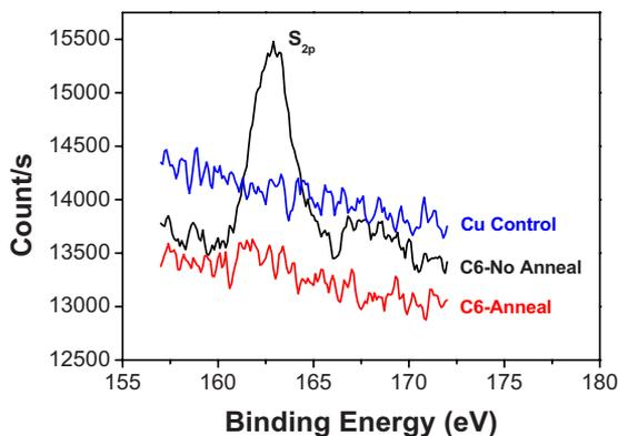
FIG. 2. (Color online) XPS data showing S content on wafer surface. Thermal desorption by annealing removes SAM.
