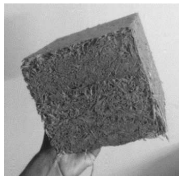
Figure 9. The bio-brick was allowed to dry in air for a month
