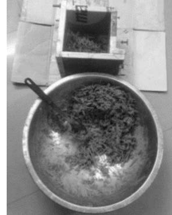
Figure 7. Chopped bagasse, lime, water and stone dust were mixed properly
