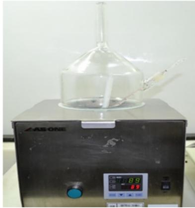
**Figure 1** Constant temperature bath for anisotropic etching
