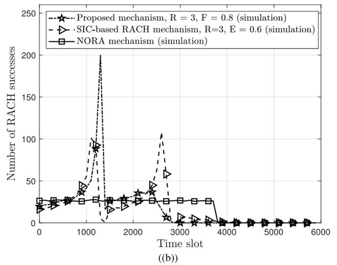
FIGURE 7. (a) Number of RACH accesses and (b) the corresponding RACH successes made in a time slot for NORA, SIC-based RACH mechanism, and the proposed SIC-NORA mechanism with  $T = 1482$ ,  $k = 54$ ,  $E = 0.6$ ,  $F = 0.8$ , and  $R = 3$ .
