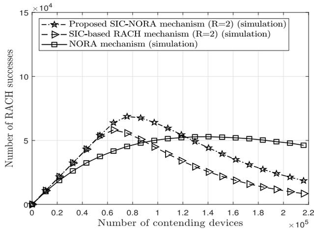
**FIGURE 8.** Number of RACH successes made in a radio frame for NORA, SIC-based RACH mechanism, and the proposed SIC-NORA mechanism with respect to increased number of M2M devices with  $T = 2000$  and  $k = 54$ .
