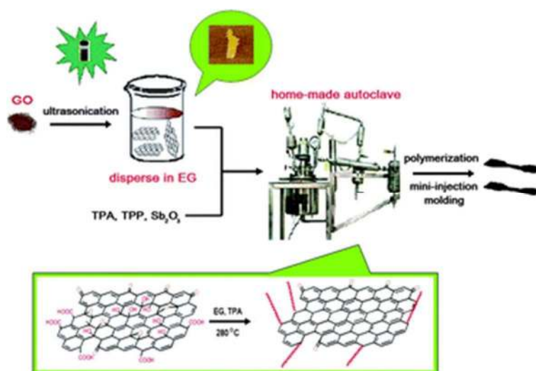
Figure 1: The synthesis of reduced polymer composite via in situ melt polycondensation (Liu et al. 29 Reproduced by the permission of The Royal Society of Chemistry).
