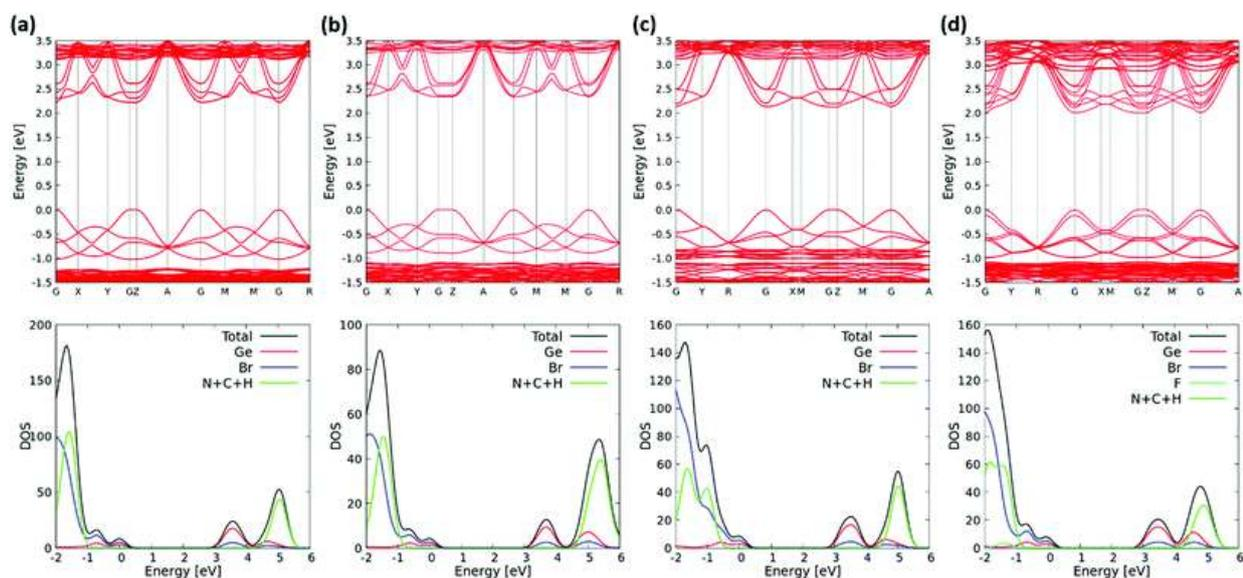
**Fig. 6** Band structure (GGA-PBE level) and DOS (HSE06-SOC level) of (a)  $\text{BZA}_2\text{GeBr}_4$ , (b)  $\text{PEA}_2\text{GeBr}_4$ , (c)  $\text{BrPEA}_2\text{GeBr}_4$  and (d)  $\text{FPEA}_2\text{GeBr}_4$ . The VBM has been set to zero in both the band structure and DOS figures.
