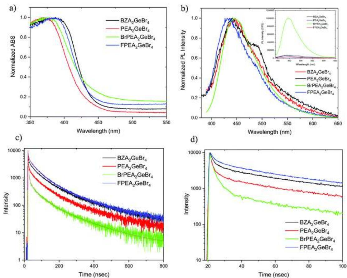
**Fig. 5** (a) Normalized optical absorbance and (b) steady-state PL ( $\lambda_{\text{exc}} = 370$  nm) and (c and d) TR decay profiles of  $\text{PEA}_2\text{GeBr}_4$ ,  $\text{BrPEA}_2\text{GeBr}_4$ ,  $\text{FPEA}_2\text{GeBr}_4$  and  $\text{BZA}_2\text{GeBr}_4$  ( $\lambda_{\text{exc}} = 375$  nm). The fitting curves are reported as solid lines in the decay measurements. The non-normalized PL spectra are shown in the inset of (b).
