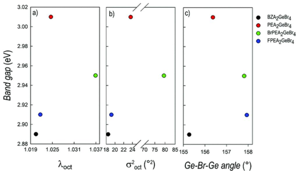
**Fig. 7** Variation of the band gap as a function of the (a) octahedral elongation, (b) angle variance, and (c) Ge–Br–Ge angle for BZA<sub>2</sub>GeBr<sub>4</sub>, PEA<sub>2</sub>GeBr<sub>4</sub>, BrPEA<sub>2</sub>GeBr<sub>4</sub> and FPEA<sub>2</sub>GeBr<sub>4</sub>.
