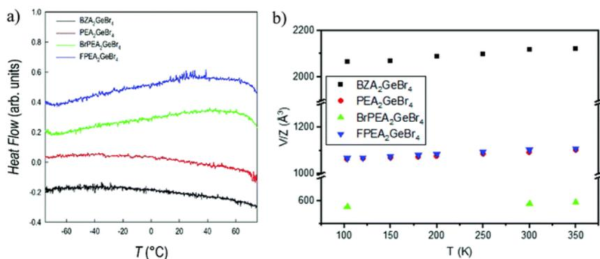
**Fig. 4** (a) DSC traces and, (b) trend of lattice volume as a function of temperature for  $\text{PEA}_2\text{GeBr}_4$ ,  $\text{BrPEA}_2\text{GeBr}_4$ ,  $\text{FPEA}_2\text{GeBr}_4$  and  $\text{BZA}_2\text{GeBr}_4$ .
