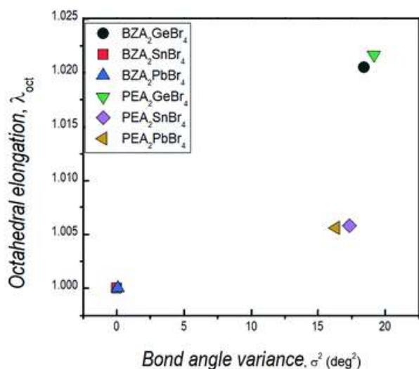
**Fig. 8** Variation of the octahedral elongation vs. bond angle variance for  $\text{BZA}_2\text{BBr}_4$  and  $\text{PEA}_2\text{BBr}_4$ , B = Pb, Sn, and Ge.
