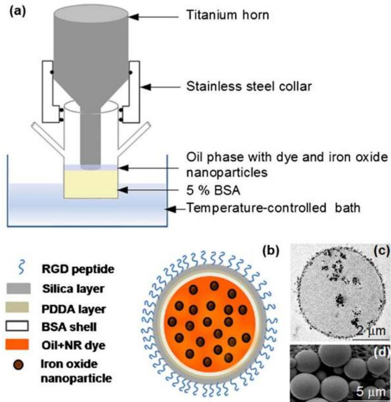
**Fig. 1.** Multimodal multifunctional protein-shell microspheres. **a** Sonication apparatus for the synthesis of protein microspheres. **b** Schematic representation, **c** TEM, and **d** SEM of protein microspheres.
