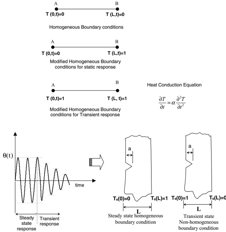
**Fig. 2** Steady state and transient response with respective modified boundary conditions.
