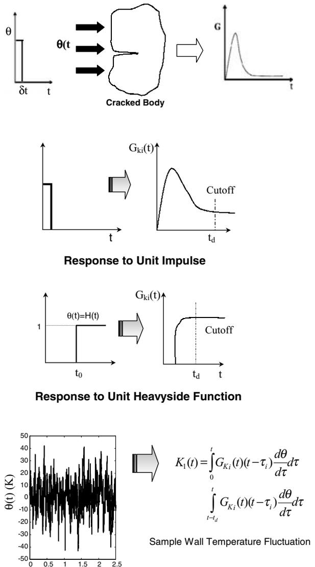
Fig. 1 Concept of Green's function approach for calculation of SIF (Lee *et al.*)
