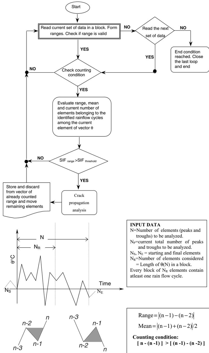
Fig. 4 (a) Flow chart for rainflow technique. (b) Illustration for rain flow technique.
