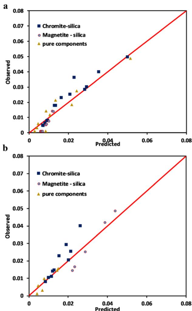
**Fig. 4** a Comparison of the experimental and predicted data set for the relative viscosity of the mixture data set used for the model building b validation of the predicted data with new experimental data set
