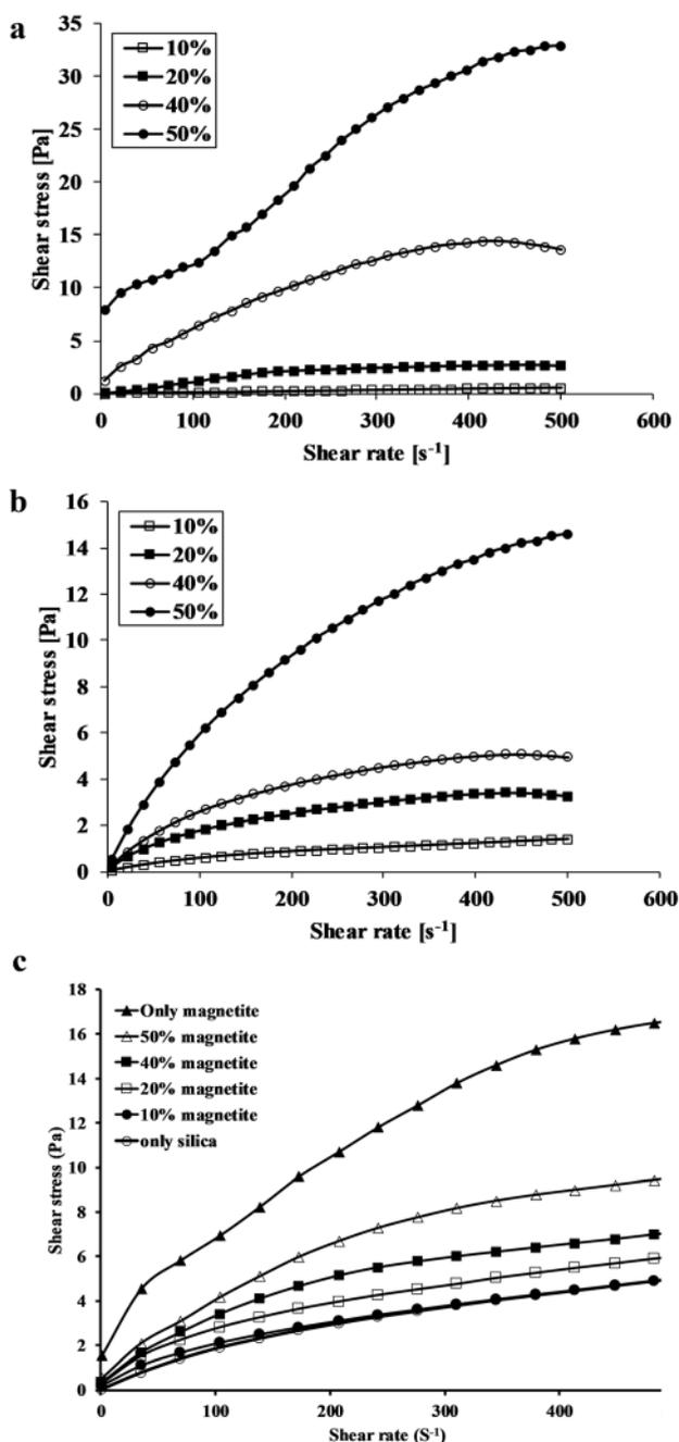
**Fig. 2** Illustration of rheograms of poly-dispersed—mono-density particles **a** pure Magnetite and **b** pure silica **c**, a CSR rheograms of magnetite and silica at various proportions of magnetite and 50 wt% total solids
