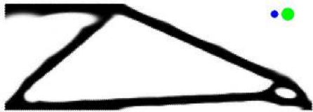
(c) Example II: cs = 0.28 units. min_{l_s} = 4cs units, max_{l_s} = 7cs units. Post optimization, \Phi = 1814.7 , g_{min}(\rho) = 49.79 , g_{max}(\rho) = 48.9 , vf = 0.26 ;
