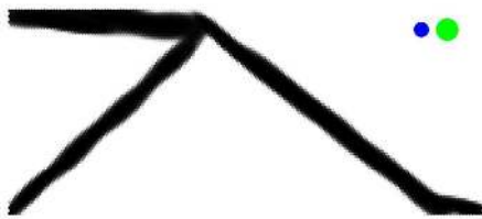
(a) Example I: cs = 0.38 units. min_{l_s} = 4cs units, max_{l_s} = 7cs units. Post optimization, \Phi = 654.1 , g_{min}(\rho) = 37.4 , g_{max}(\rho) = 35.3 , vf = 0.35 ; BWI = 0.06 .
