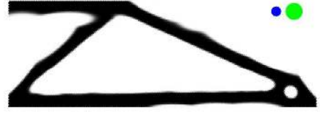
(b) Example II: cs = 0.28 units. min_{l_s} = 4cs units, max_{l_s} = 7cs units. Post optimization, \Phi = 1462.7 , g_{min}(\rho) = 81.8 , g_{max}(\rho) = 78.8 , vf = 0.33 ; BWI = 0.04 .
