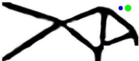
(g) Example IV: cs = 0.38 units. min_{l_s} = 4cs units, max_{l_s} = 6cs units. Post optimization, \Phi = -0.068 , g_{min}(\rho) = 86.00 , g_{max}(\rho) = 70.44 , vf = 0.29 ;
