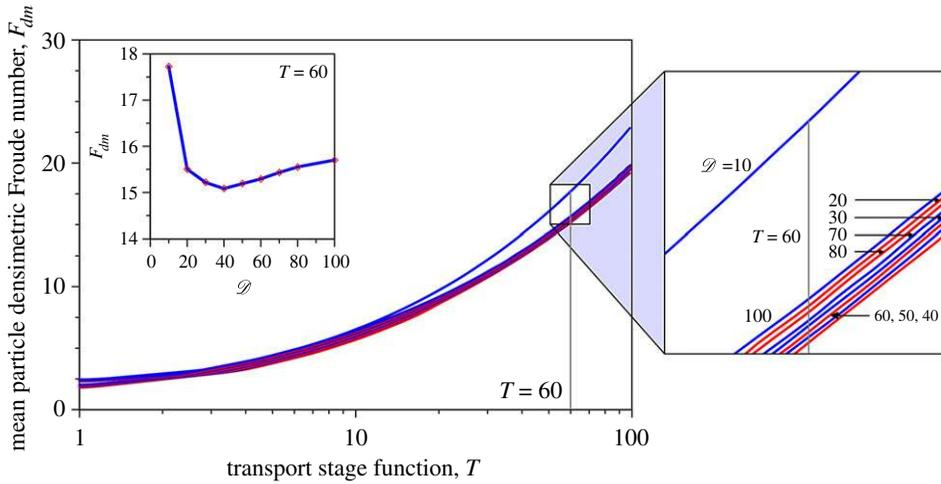
**Figure 8.** Mean particle densimetric Froude number  $F_{dm}$  versus transport stage function  $T$  for different values of particle parameter  $\mathcal{D}$ . In the inset, the variation of mean particle densimetric Froude number  $F_{dm}$  with particle parameter  $\mathcal{D}$  at a transport stage function  $T$  of 60 is shown. (Online version in colour.)
