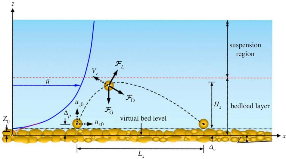
**Figure 1.** Conceptual sketch of bed particle saltation in turbulent wall-shear flow.
