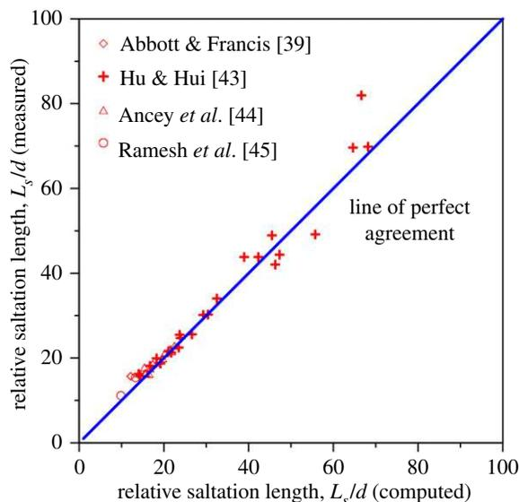
**Figure 6.** Computed versus measured relative saltation length  $L_s/d$ . (Online version in colour.)
