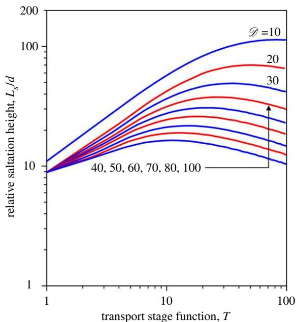
**Figure 5.** Relative saltation length  $L_s/d$  versus transport stage function  $T$  for different values of particle parameter  $\mathcal{D}$ . (Online version in colour.)
