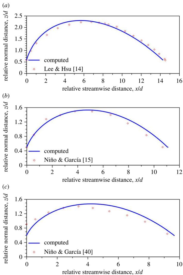
**Figure 2.** Comparison of the bed particle trajectories obtained from this study with the experimental data for (a)  $d = 1.36$  mm, (b)  $d = 0.67$  mm and (c)  $d = 0.56$  mm. (Online version in colour.)
