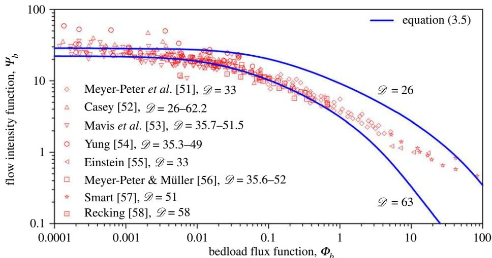
**Figure 10.** Bedload flux function  $\Phi_b$  versus flow intensity function  $\Psi_b$ . (Online version in colour.)
