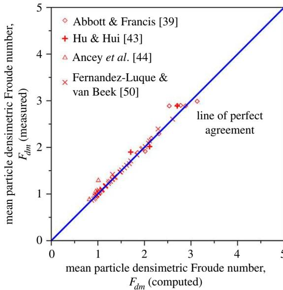
**Figure 9.** Computed versus measured mean particle densimetric Froude number  $F_{dm}$ . (Online version in colour.)
