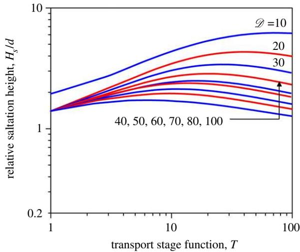
**Figure 3.** Relative saltation height  $H_s/d$  versus transport stage function  $T$  for different values of particle parameter  $\mathcal{D}$ . (Online version in colour.)
