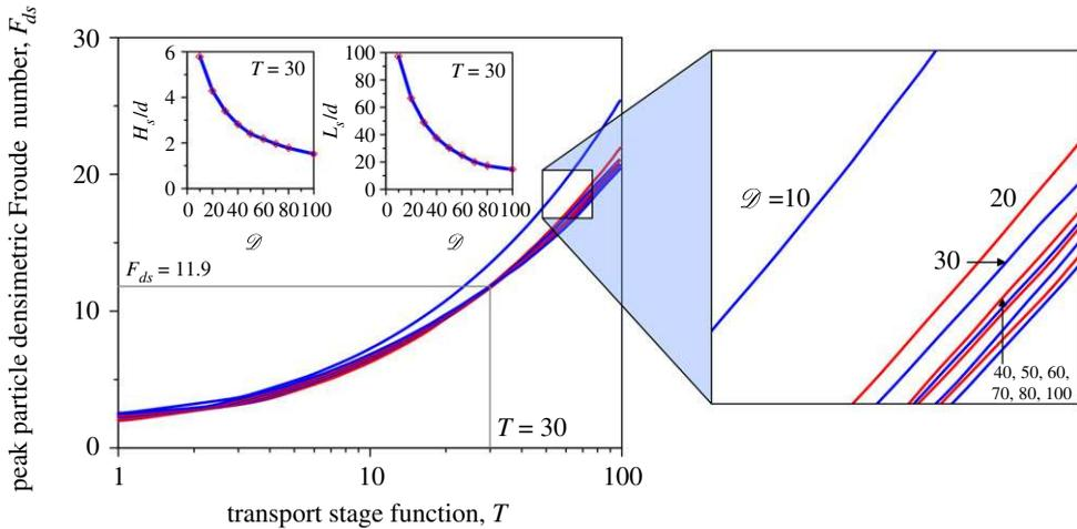
**Figure 7.** Peak particle densimetric Froude number  $F_{ds}$  versus transport stage function  $T$  for different values of particle parameter  $\mathcal{D}$ . In the inset, the variations of relative saltation height  $H_s/d$  and relative saltation length  $L_s/d$  with particle parameter  $\mathcal{D}$  at a transport stage function  $T$  of 30 are shown. (Online version in colour.)
