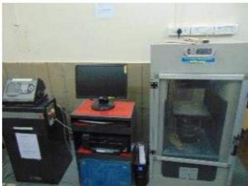
(a) Controls Compression Testing Equipment
