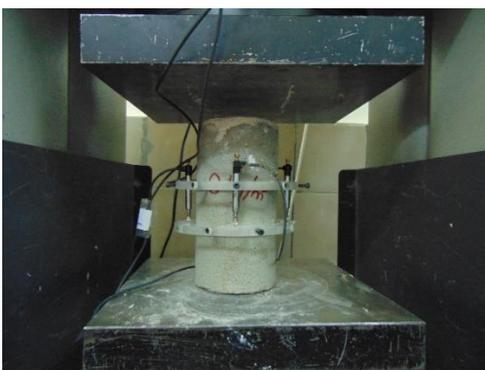
(c) Testing set-up with LVDTs
