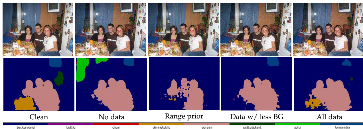
Fig. 12. Sample failure case for the semantic segmentation using the FCN-8s-VGG model. Top row shows the clean and corresponding perturbed images for no prior to various priors. Bottom row shows the predicted segmentation maps. Note that the people segments are undisturbed by the addition of various perturbations.
