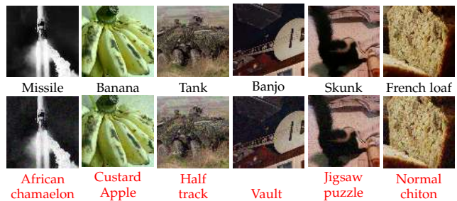
Fig. 3. Sample original and adversarial image pairs from ILSVRC validation set generated for VGG-19. First row shows original images and corresponding predicted labels, second row shows the corresponding perturbed images along with their predictions.
