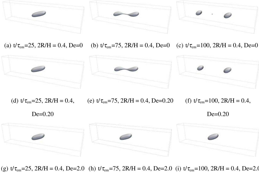
FIG. 3: Deformation/Break-up after the startup of a shear flow with confinement ratio 2R/H = 0.4 . We report the time history of droplet deformation and break-up including 3 time frames which represent, in the Newtonian case ( De = 0 ), initial deformation (left column, t = 25\tau_{em} ); deformation prior to break-up (middle column, t = 75\tau_{em} ); post-break-up frame (right column, t = 100\tau_{em} ). We use the emulsion time \tau_{em} (see Eq. (8)) as a unit of time. The second row of images is related to a weakly viscoelastic droplet ( De = 0.2 ), indicating that non-Newtonian properties do not affect the droplet deformation and break-up much. The third row of images is related to a viscoelastic droplet with Deborah number above unity ( De = 2.0 ), and indicates that non-Newtonian properties stabilize the droplet deformation and inhibit droplet break-up. Note that the Capillary number is kept fixed to the post-critical Newtonian value Ca = 0.34 , which is the smallest Capillary number available for us at which we observe break-up in the Newtonian case. In all cases, the viscous ratio between the droplet phase and the matrix phase is kept fixed to \lambda = \eta_D/\eta_M = 1 , independently of the degree of viscoelasticity. The finite extensibility parameter is fixed to L^2 = 10^2 .
