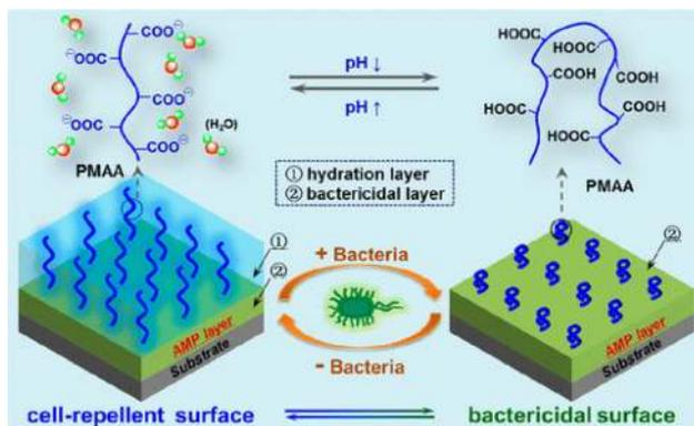
**Figure 11** pH-responsive switchable antibacterial surface using AMP and PMAA. Adapted with permission from Ref. [111] Copyright (2016) American Chemical Society.
